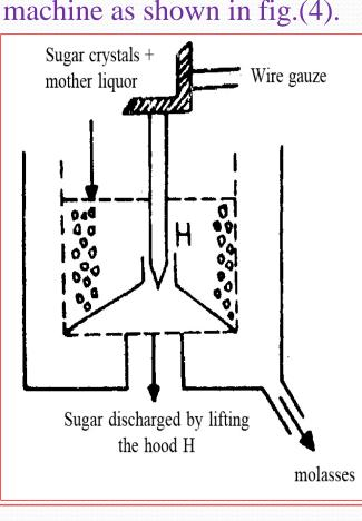
A centrifugal machine composed of cylindrical basket suspended on a "spindle" has perforated sides lined with wire cloth. The machine revolves at a speed from 1000 to 1800 rpm. The perforated lining retains the sugar crystals. While, the mother liquor (molasses) passes through lining because of the centrifugal force exerted. The sugar crystals are carefully washed by injecting a fine spray of water or by means of jet of steam and air, to remove last traces of molasses still sticking them.
