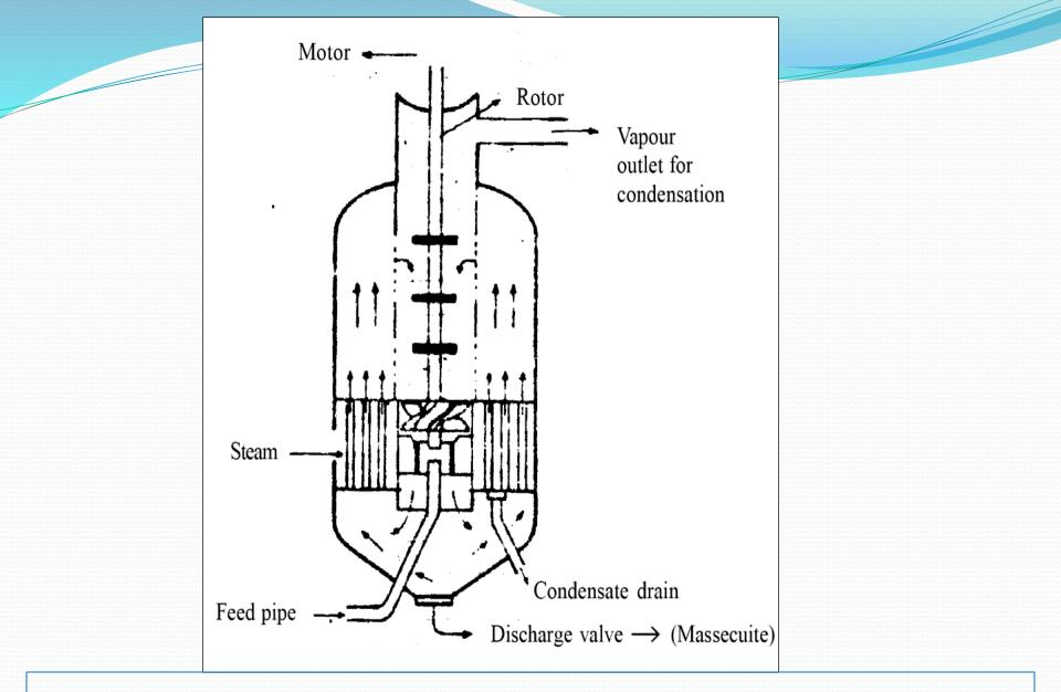
The crystallization of sucrose in vacuum pan is called as 'Sugar boiling" and each boiling is termed a 'strike'.
