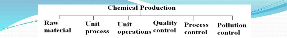
In order to get maximum yield, the chemical process is designed in a particular way. The raw materials are given physical treatment involving unit operations such as heat transfer, mixing, filtration, solvent extraction, etc. Then in a reactor, chemical treatment is given by which transformation occurs. The products are then further treated physically for the separation and purification in order to get a desired product. A typical chemical process is as follows:
